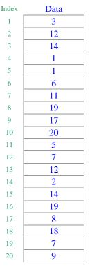
The "linear search" method starts looking for the required element at the very "top" of the array (i.e. at the *first* element).
