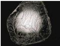
A fractal is formed when pulling apart two glue-covered acrylic sheets.
