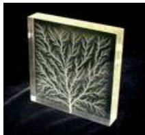
High voltage breakdown within a 4" block of acrylic creates a fractal Lichtenberg figure.
